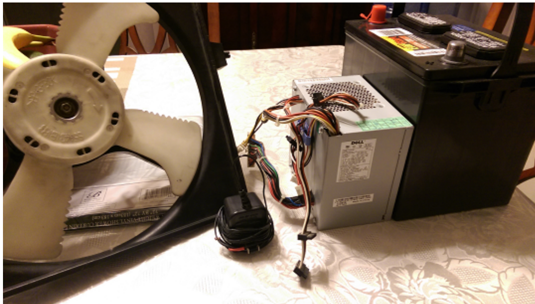
Figure 4: 9V adapter, PC power supply, 12V car battery for power to the fan.
